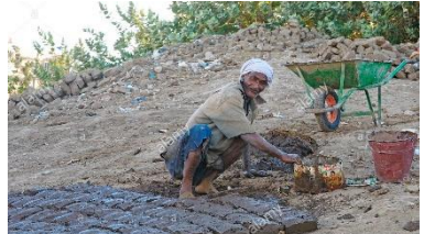
Figure 2: The making of mud bricks from the Black soil of 3bw (Elephantine) island
